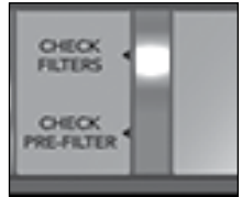
Fig. 7 Will illuminate when it is time to change HEPA filters
