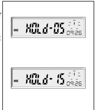
During the lockout period, if battery is removed the system will enter 15-minute lockout period.
