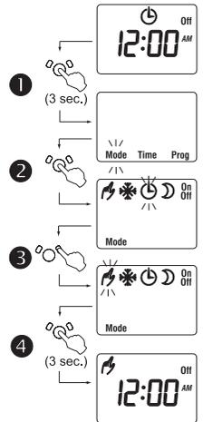
**NOTE:** The timer automatically returns to its normal display if you do not press any button for 60 seconds.
