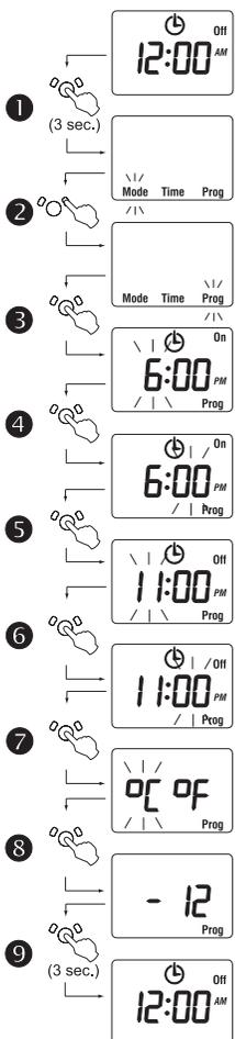
**NOTE:** The timer automatically returns to its normal display if you do not press any button for 60 seconds.
