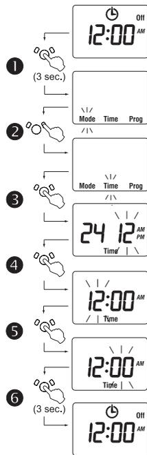
**NOTE:** The timer automatically returns to its normal display if you do not press any button for 60 seconds.
