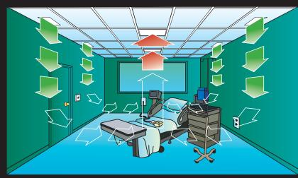
The F120 unit is designed for hospital applications as well. The modular design of the air supplies and returns allow maximum flexibility when planning the appropriate air recirculation pattern to maximize the overall system performance. The filtered air exits the unit at ceiling height, producing a coanda air flow pattern that helps push filtered air efficiently past the breathing zone and back to the Hepa-Flow CPZ™ return module.
